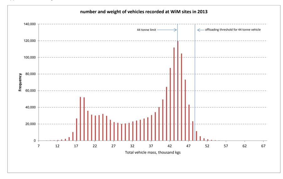
Appendix Four: Weigh-in-motion data for 8 axle truck and trailer combinations
